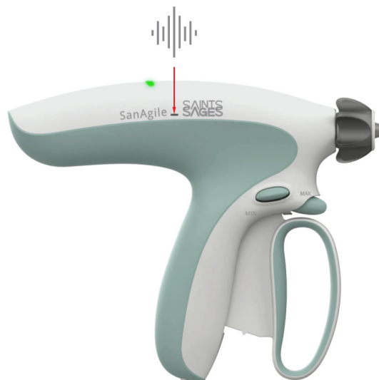
Figure 4: Dissector Status LED Illuminates Green and Audio Tone Beeps
